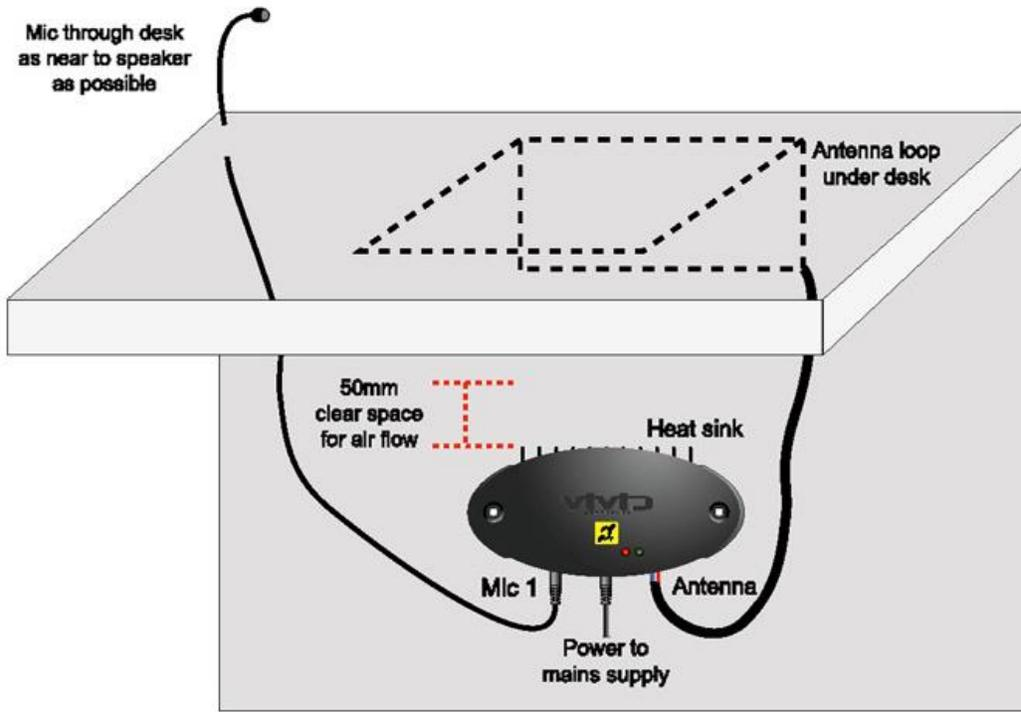
Ensure that the RED power indicator light is lit. If yes, continue to step 6. If not, make sure the power supply is plugged into an active power outlet and that the power supply is plugged into the amplifier. If the RED power indicator light is still not lit, Contact Advanced Listening Systems at 1-250-580-2180.
